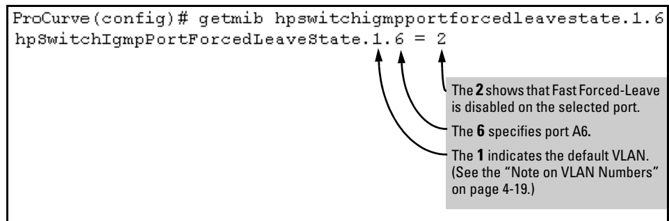
Figure 4-5. Example Listing the Forced Fast-Leave State for a Single Port on the Default VLAN
